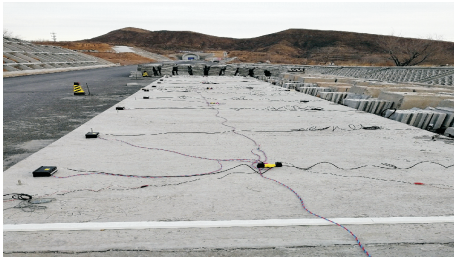
图3 埋设监控点及拉线传感器布置
